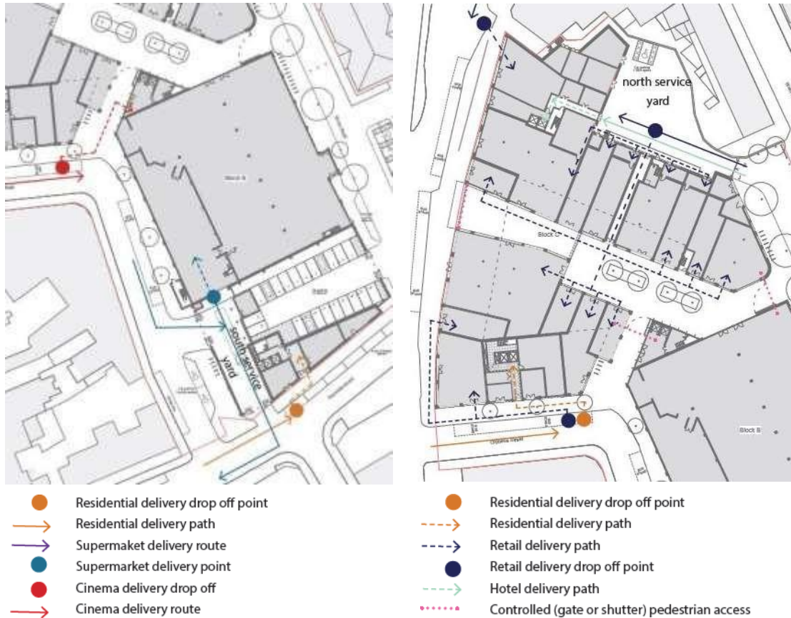
Figure 54 (above left): Block B delivery strategy. Figure 55 (above right): Block C delivery strategy.
