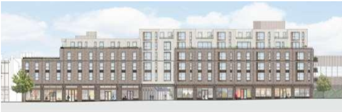
Figure 18 (above): West elevation of Block C, showing the ground level active frontage extending the full length of the façade, broken only by the canopied opening into the new shopping street.
