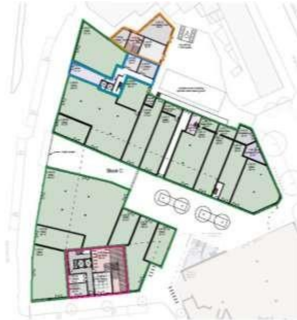
Figure 17 (above): Block C ground floor layout. The retail uses are edged in green, the residential core in pink, the hotel entrance in blue and shared retail/hotel ancillary spaces in orange.
