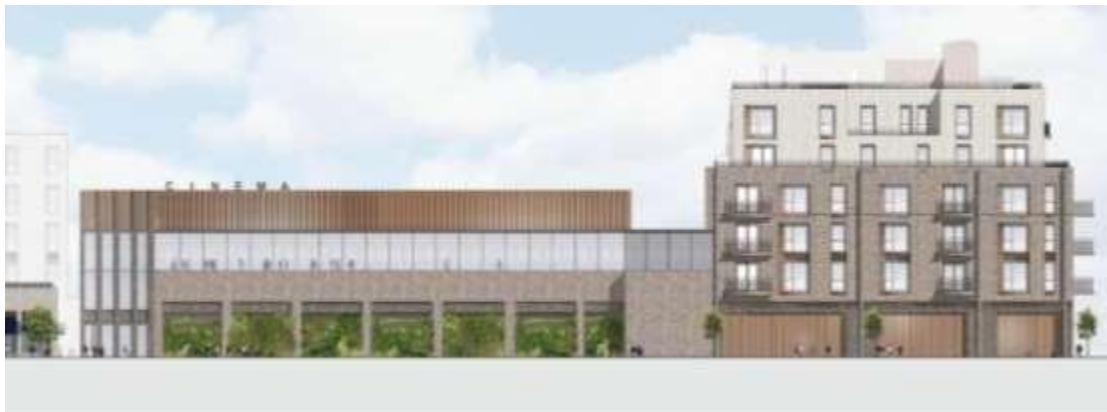
Figure 14 (above): West elevation of Block B, showing how the cinema space would sit above the retained supermarket (remodelled on its rear façade with greening) and its relationship to the proposed residential block on the southern part of Zone B.
