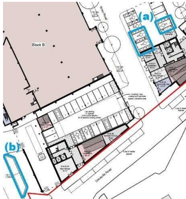
Figure 53: Plan showing the proposed parking provision, with (a) denoting the three dedicated residential spaces and (b) denoting the on-street publicly-accessible Blue Badge spaces.
